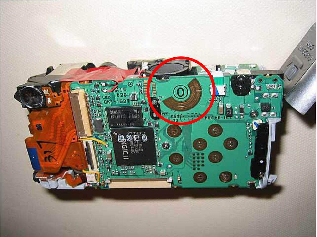
You may have already deduced what we need to do. The first is to clean the brushes and circuit dial of any visible gunk that may have accumulated on them. I recommend a Q-tip, very slightly dampened with a drop of alcohol. Be careful with the alcohol, you don't want it running all over the circuit board. Remember to check and clean off any residual cotton hairs/lint from the Q-tip on both of these components. A little compressed air blowing would help here.
